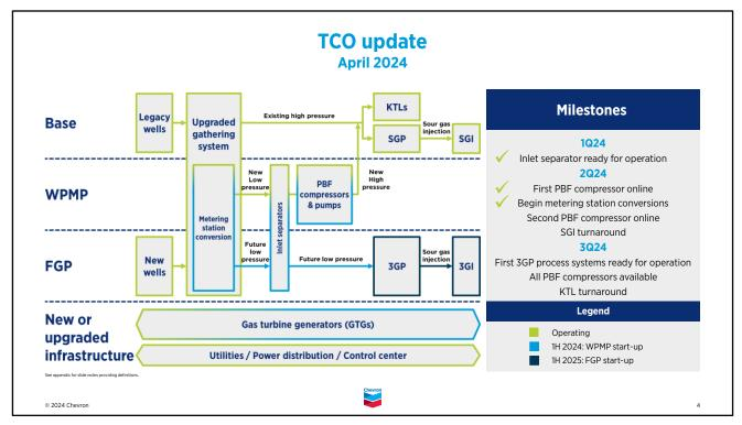
At TCO, we achieved start-up of WPMP this month with the first inlet separator and pressure boost compressor in service and conversion of the first metering station to low pressure.
